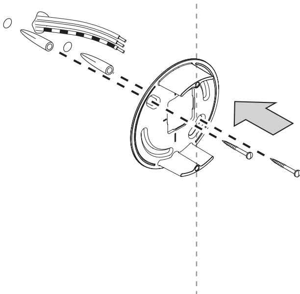
Cut the mains cable to a length of 5 cm and strip the insulation from the ends.
