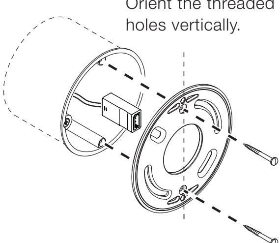
Screw the mounting plate to the hollow ceiling box. As you do so, guide the socket of the LED connection cable through the opening.
