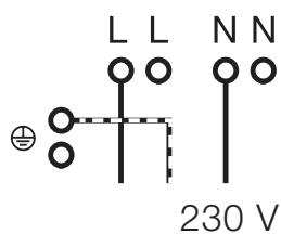
Connected with through-wiring
