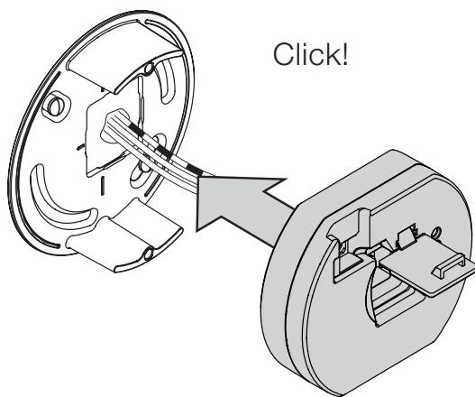
Lock the converter into the mounting plate so that it is fitted flush.
