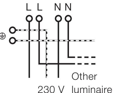
Connect the ends of the mains cable to the converter terminals in accordance with the diagram.
