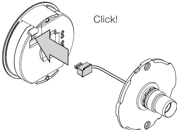
Insert the plug of the luminaire body into the socket of the converter.
