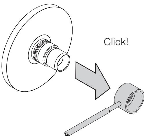
Remove the carbon rod from the body (not necessary for the version with fixing ring).
