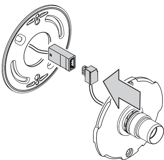
Connect the plug of the body to the socket of the LED connection cable.
