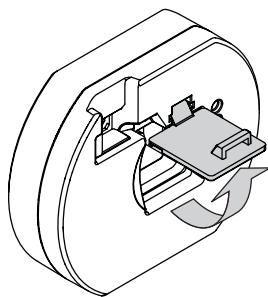
Using a screwdriver, open the flap in the middle of the converter.
