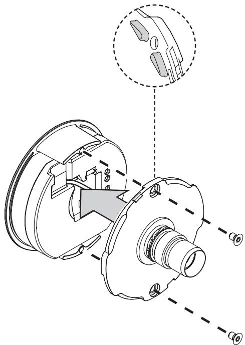
Lay the cable in the recess of the converter. Do not trap the cable.
