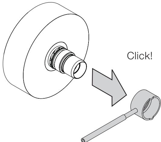
Undo the cover by turning it anti-clockwise and remove it.
